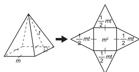
$$\begin{aligned} \text{Luas permukaan/ Surface area} \\ = m^2 + \left(4 \times \frac{1}{2}mt\right) \\ = m^2 + 2mt \end{aligned}$$
